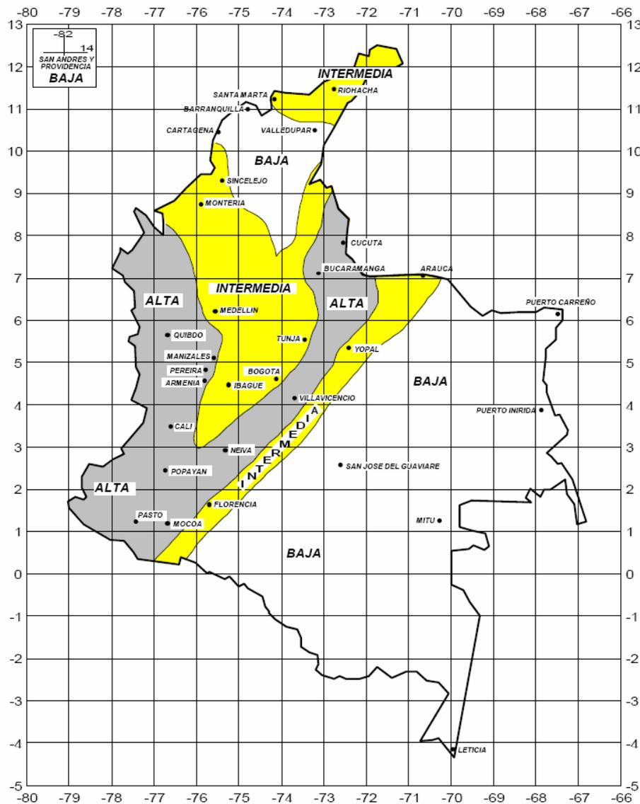
Figure 3.1. Colombian seismic hazard map
