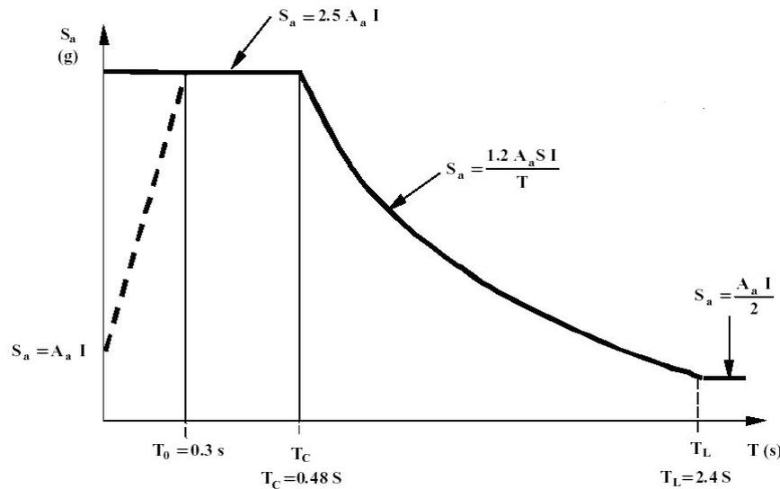
Figure 3.2. Elastic Design Spectrum (NSR-98).
