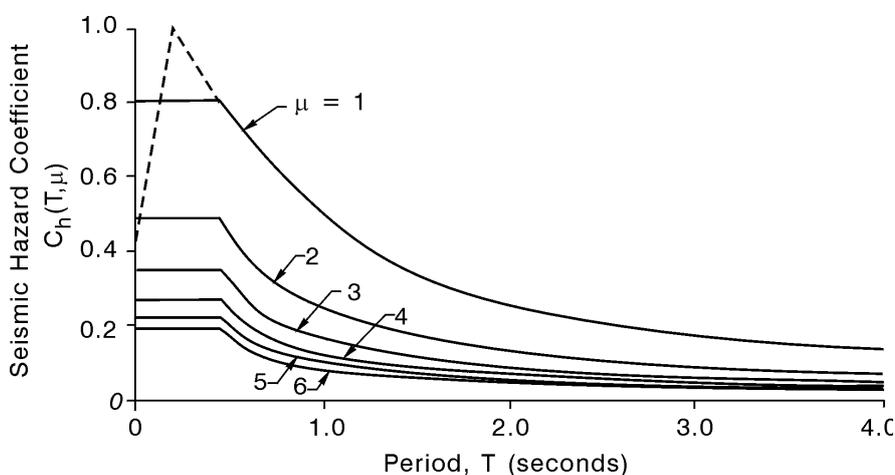
Figure 5.1. Estimation of the required structure ductility factor  $\mu_{sd}$
